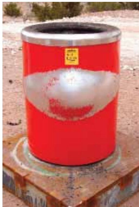
Post Detonation: Close-up of featured test photo – American Innovations Protector Model Bomb Receptacle. Notice the construction of the test stand used during this testing.
